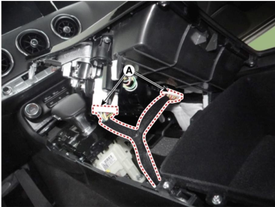
4. Remove the connector (A) from the console floor switch complete.
