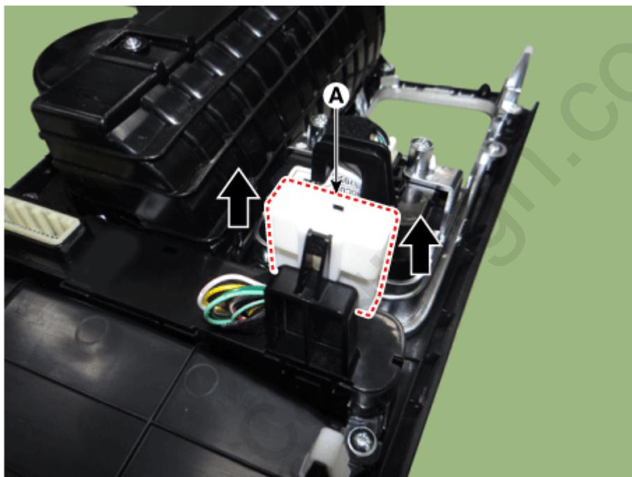
5. Remove the console floor switch complete (A) after loosening the mounting screws.
